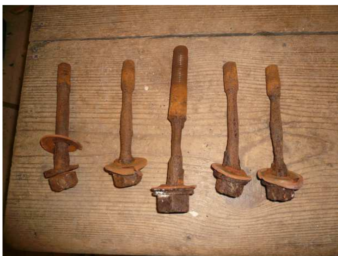
Five of the 1903 head bolts removed by Whites
